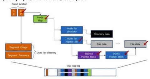
F2FS Index Structure: Indirection and Multi-Headc Logs Optimize Updates
